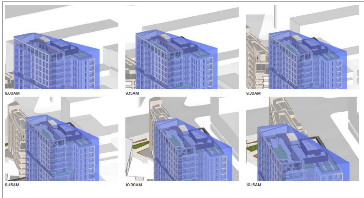
Figure 4. D1A Tower Lift-Overrun Breach
